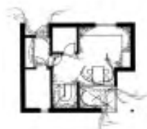
Border space. Hestra. Marked in heavy lines on a 4 BR apartment's entry level. Scale 1:400.
