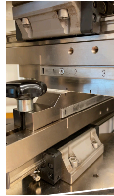
Figure 2: Fixture for ZD-tests.
