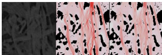
Figure 1: X-ray computed tomography scan (right), simulation result (middle), predicted with generative adversarial network (left).
