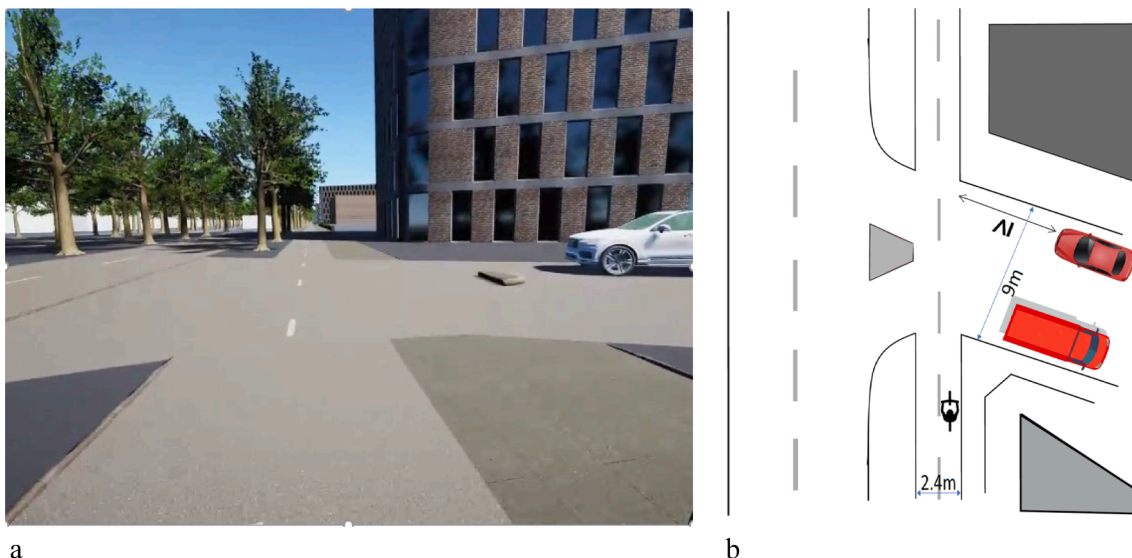
Fig. 2. Layout of the intersection simulated in the experiment; (a) cyclist view of the intersection, (b) top view of the intersection.
