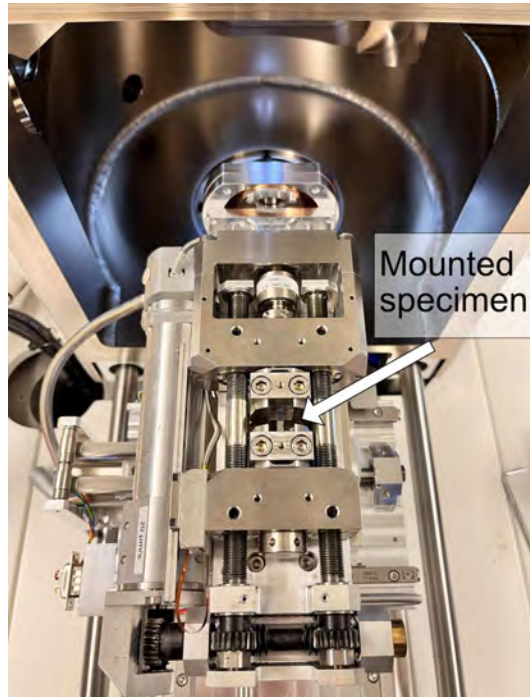
Figure 3.17: In-situ tensile stage with mounted SENT specimen.
