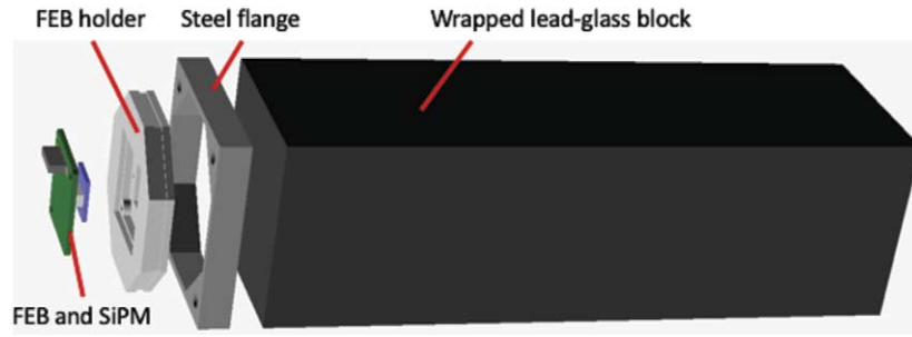
Fig. 58. Exploded view of an LEC lead glass counter.
