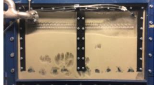
(b) 0.6 m/s, V_{sv} \sim 30\% , VD Mode 1B with Internal baffles, AD 1660
