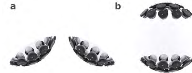
Figure 3.1: Array configurations of an acoustic levitator of a) single-side independent arrays, and b) coupled arrays forming a cavity.
