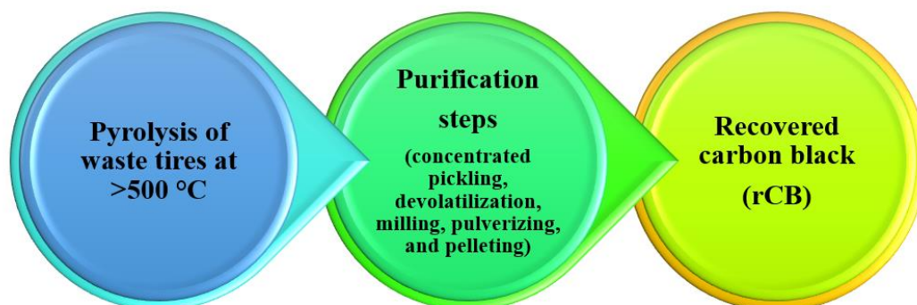
Figure 18. Overview of the general steps in rCB production from waste tires.
