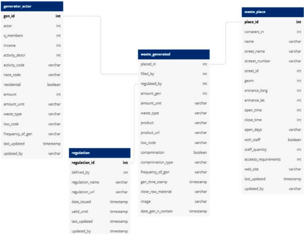
Fig. 12.. Relational data model schema for waste transfers.
