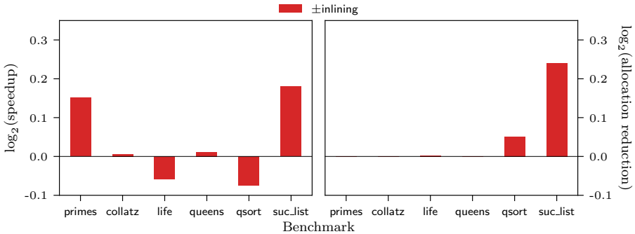
Fig. 3. Graphs showing the performance impact of our inliner: the base-2 logarithm of a ratio of measurements (execution time or heap allocations) with/without the inliner enabled: \log_2(m_{\text{disabled}}/m_{\text{enabled}}) . Error bars are too small to be visible.
