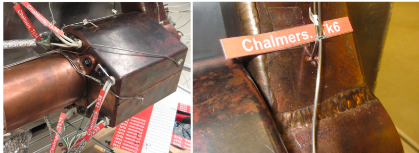
Fig. 3. Examples of thermocouples embedded into catalyst and the exhaust pipe.
