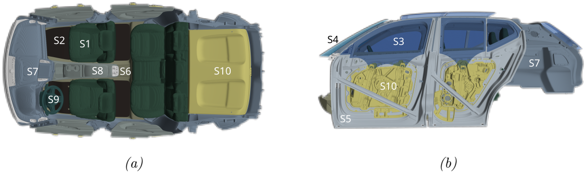
Figure 3.1: Cabin solids colored based on the corresponding material property from Table A.1 in Appendix A (a) Top view; (b) Side view.
