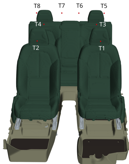
Figure 3.13: Positions of thermocouples (T1-T8) placed in the car during experiments.
