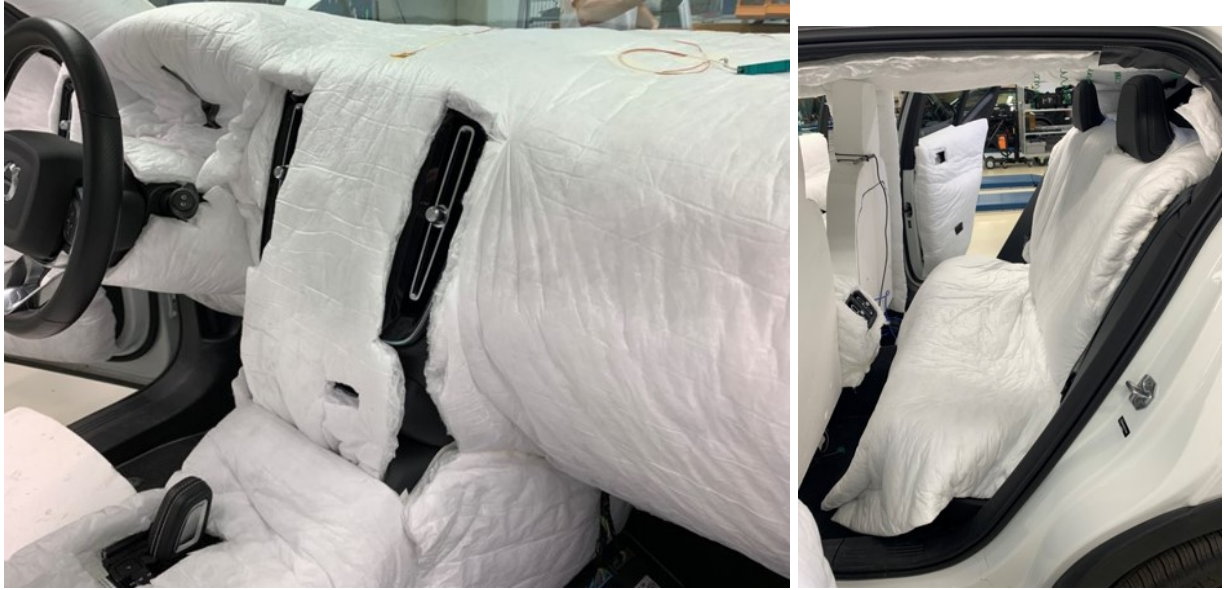
Figure 3.12: Experimental setup of the fully insulated cabin.
