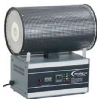
Figure 4.1: Tubular furnace used for the single-atmosphere exposures and Cr(VI) evaporation measurements.
