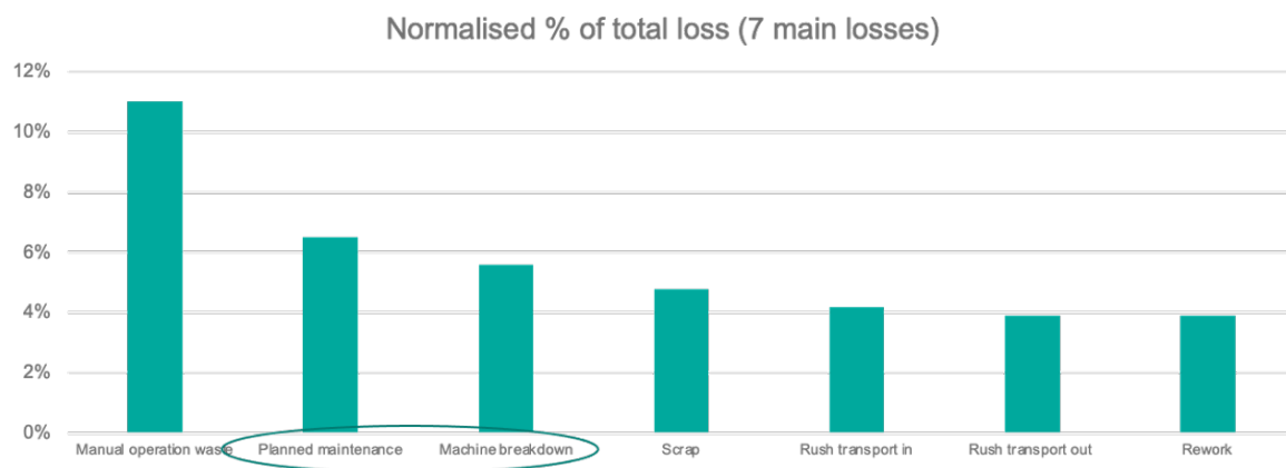
Figure 35: Maintenance losses are a significant contributor to the top losses
