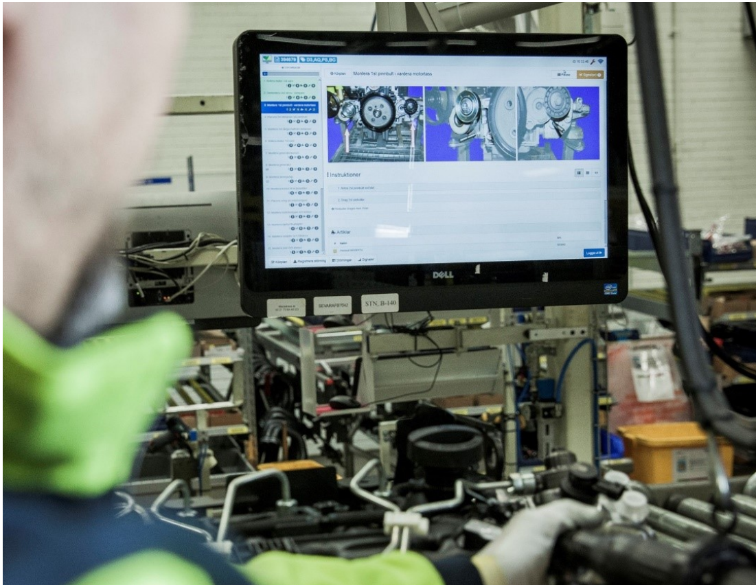
Figure 12. Digital instructions with confirmation in Casat from H&D Wireless AB. Photo reproduced with permission from H&D Wireless AB.
