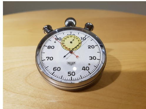
Figur 10. Picture of a stopwatch used in the past with so-called centiminute, meaning a minute is divided into one hundred parts. A base of one hundred makes it easier to do mental arithmetic. Foto: Peter Almström.
