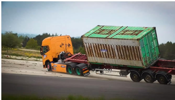
Figure 4.9: A tractor-semitrailer combination rolling over during electric truck crash safety tests [30]
