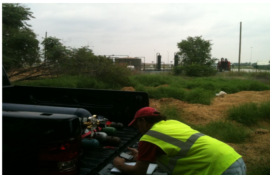
Figure 17 Tracer releases of \text{N}_2\text{O} from a car upwind of a well and mobile compressor station in Fort Worth.
