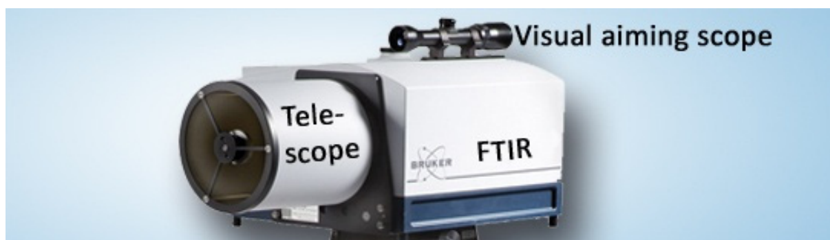
Figure 19 The passive thermal emission FTIR (Bruker Optics EM27), assembled with a infrared telescope and visual aiming scope, all mounted on a tripod.
