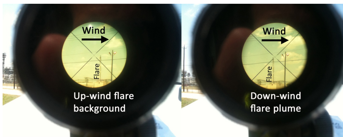
Figure 63 Thermal emission measurements of a flare exhaust plume. The down-wind flare emission signal is subtracted with the up-wind flare thermal background signal. The aiming cross is approximately the centre of the viewing infrared emission telescope.
