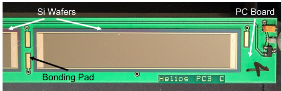
Figure 3.3: One Si PSD from the HELIOS Si array. There are electrical contacts at both short edges of the front face of each PSD (the lighter-colour part of a PSD) as well as one full-area contact at the back face. Figure from Ref. [13].
