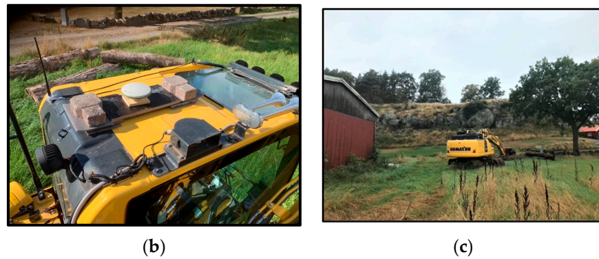
Figure 1. The experimental set up. (a) The GNSS antenna marked with a green circle on top of the excavator. (b) Top view of the excavator showing the GNSS antenna. (c) The excavator facing NW direction with the tree on the right and the house on the left.
