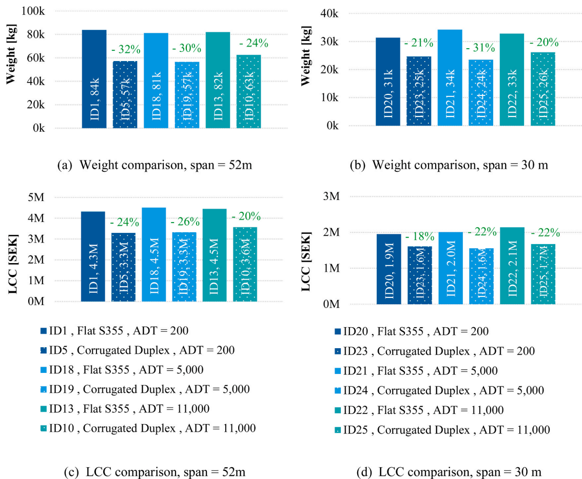
Fig. 12. Evaluation of weight and LCC potential saving for different bridge span lengths.
