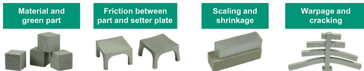
Figure 5. Categorization of influences on component design in the metal binder jetting process chain [27]. Reproduced with permission from Springer Nature.
