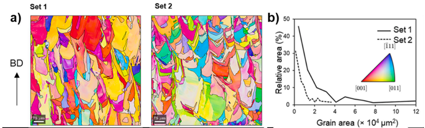
Fig. 2. (a) EBSD orientation maps along the build direction (BD) from the two sets. (b) Grain size distributions.
