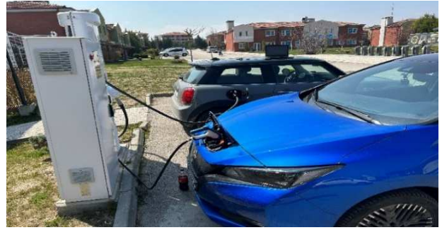
Fig. 4. Simultaneous testing of V2G and V1G compatible vehicles.
