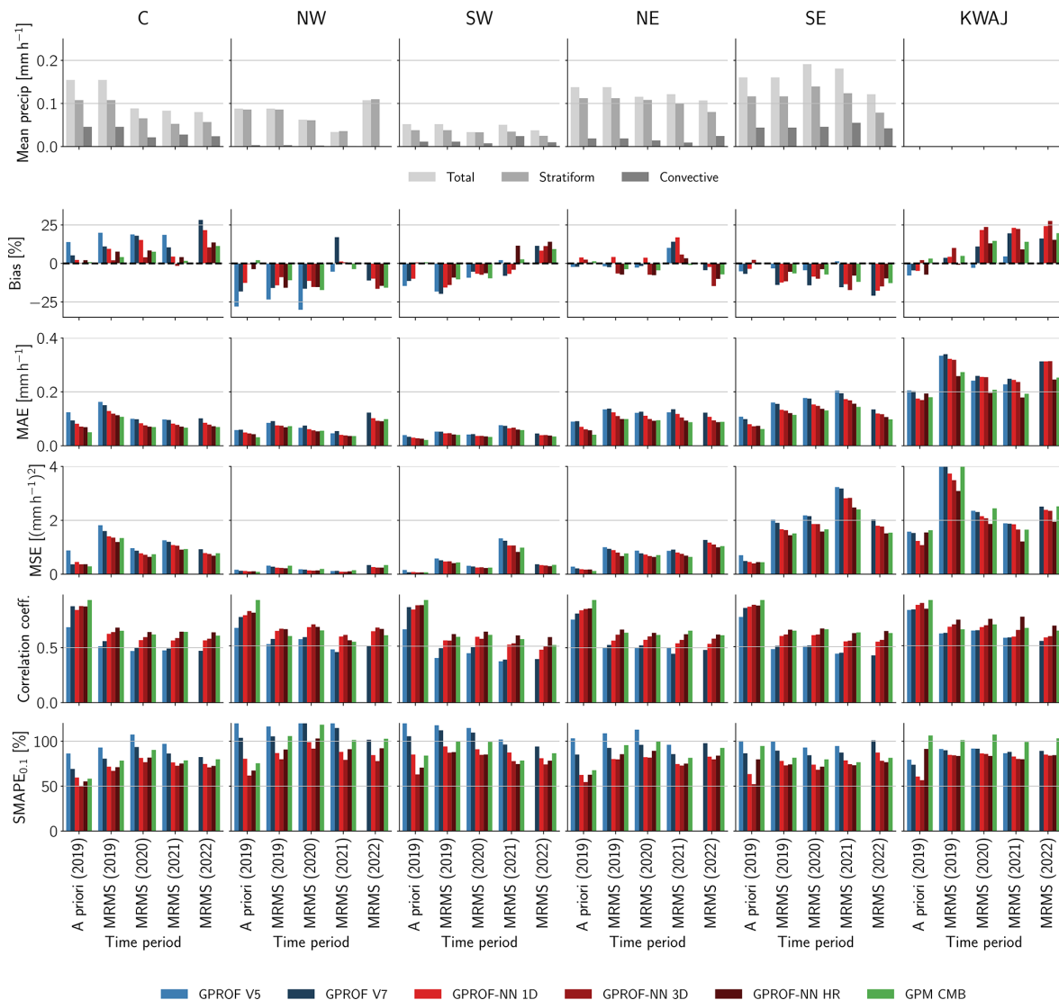
Figure 8. Retrieval accuracy metrics for the assessed climate regions over the CONUS and the tropical Pacific. The first row shows the mean precipitation rate of the reference data and, where such a classification was available, the contributions from convective and stratiform precipitation. Remaining rows show accuracy metrics for the comparison of the retrieval results against the reference and validation data. Columns from left to right show the results for the for the five considered regions.
