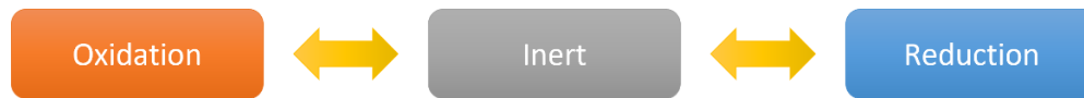
Figure 3.6 Three steps in a cycle in the fluidized bed batch reactor experiment.
