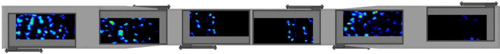
Figure 4. Illustration of the base of the Sensor Sleeper with overlaid example results for the six pressure sensors for traffic in the through route. The sensor positions correspond to Figure 2 with sensors f_{b1} - f_{b6} counted from right to left. The brighter the colour the higher the contact pressure (black = zero pressure).
