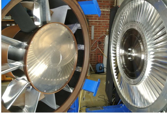
Figure 2.4: The disassembled LPT and TRS components, highlighting the modular design of the TRS.
