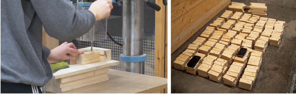
Figure A.20: To the left, the timber blocks are being drilled using a mounted drill in the wood workshop utilising a jig to avoid measurements each time. To the right, the finished timber blocks and the timber studs connecting the laths to the base plate are seen.
