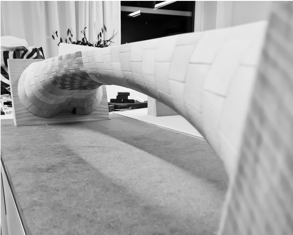
Figure 6.10: Close-up of a physical model of a single-span hydrostatic masonry bridge built during a workshop in 2022, where the cross-section at mid-span is a superellipse or Lamé curve.
