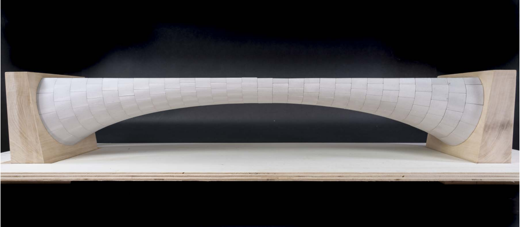
Figure C.1: Physical model of a single-span hydrostatic masonry bridge built during a workshop in 2022.
