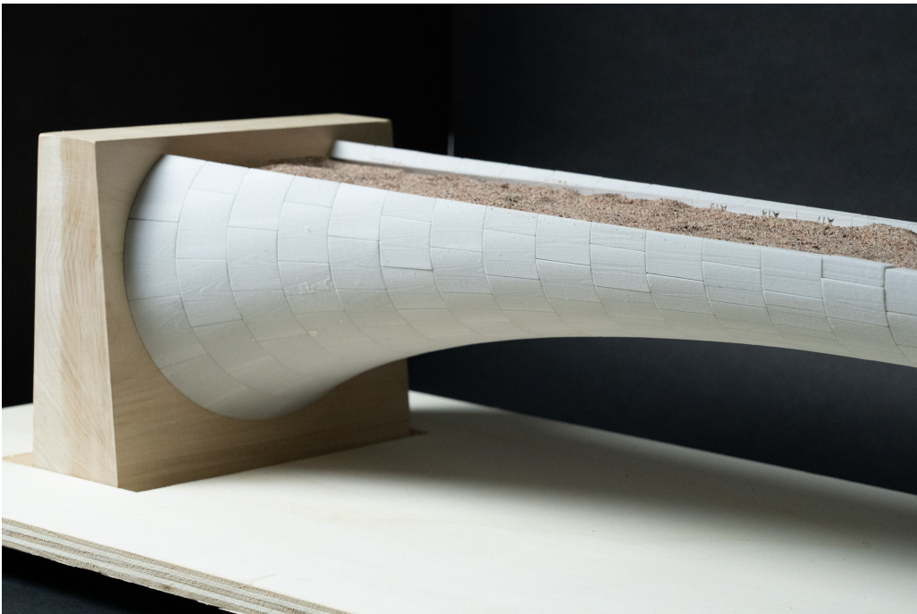
Figure C.11: Close-up of a physical model of a single-span hydrostatic masonry bridge built during a workshop in 2022.
