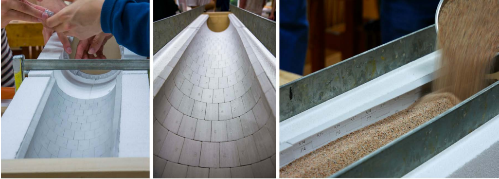
Figure C.10: Left, the assembly in progress on the false work. Middle, the bridge before adding fill. Right, adding the necessary load from fill such that the false work could be removed.
