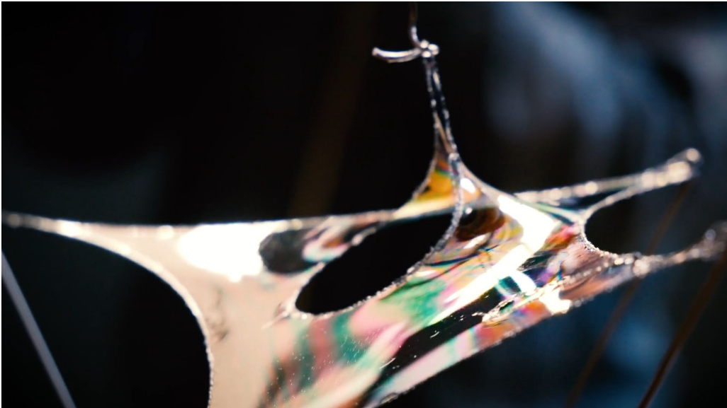
Figure 4.6: Soap film model similar to those used by Frei Otto and Sergio Musmeci, among others.
