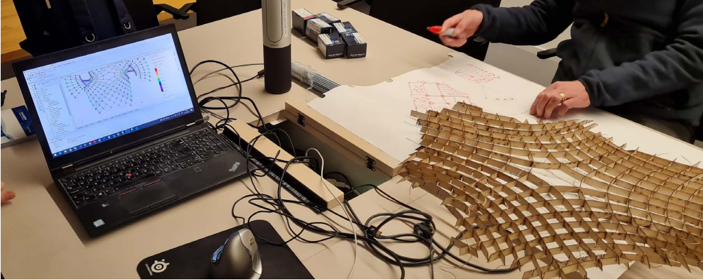
Figure B.4: Design process of the bracing pattern using a combination of drawing and reasoning, physical model tests, and structural analysis.
