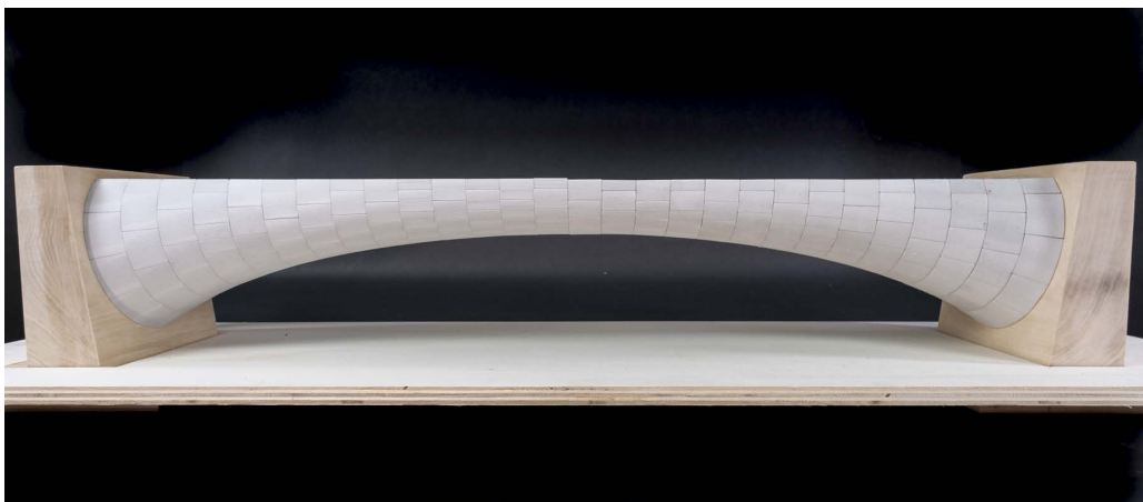
Figure 6.9: Physical model of a single-span hydrostatic masonry bridge built during a workshop in 2022.
