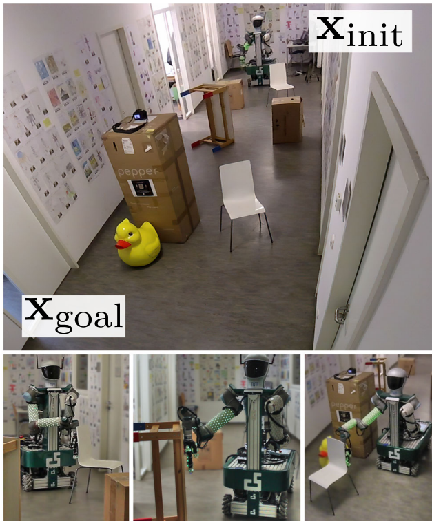
Figure 1. Navigation among movable obstacles: the robot autonomously navigates from the initial pose to the goal pose, negotiating movable and nonmovable obstacles along the way.
