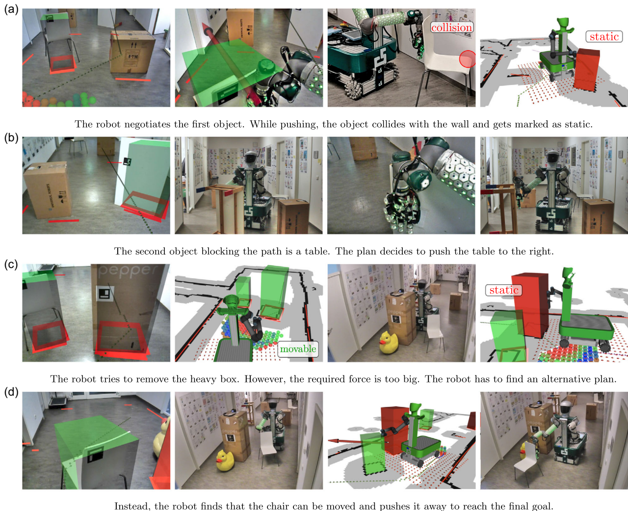
Figure 12. Experiment: key-frames of the real execution. The task is to autonomously reach the opposite side of the hallway.
