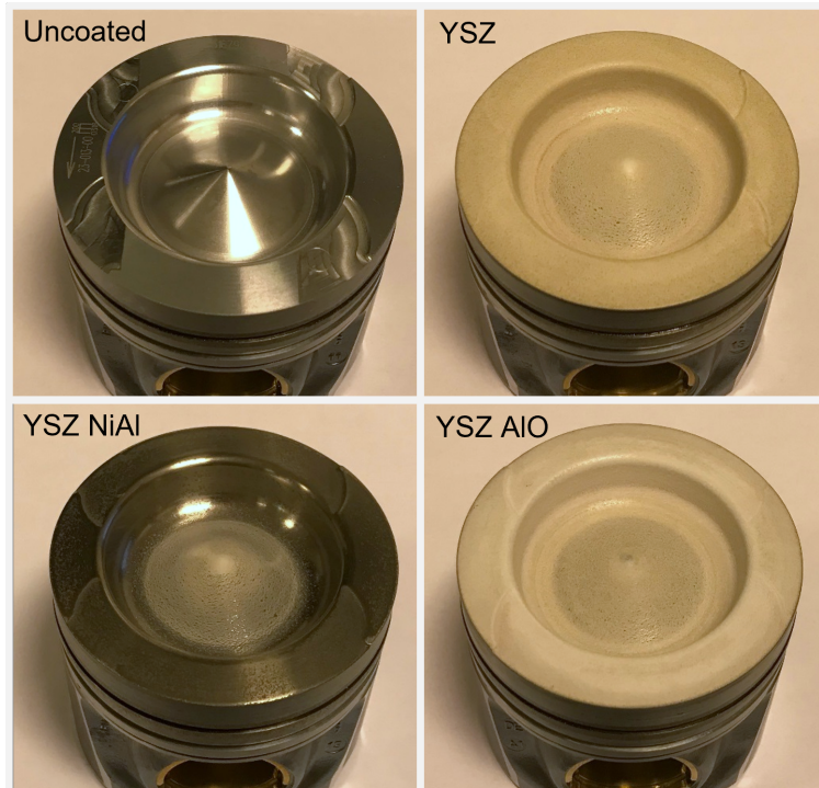
Figure 25. Uncoated reference piston and pistons coated with YSZ. The surface of the two pistons at the bottom is sealed with a nickel alloy (left) and alumina (right) layer.
