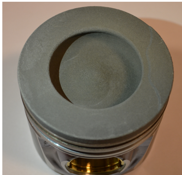
Figure 18. Piston with hard anodized aluminium oxide surface.
