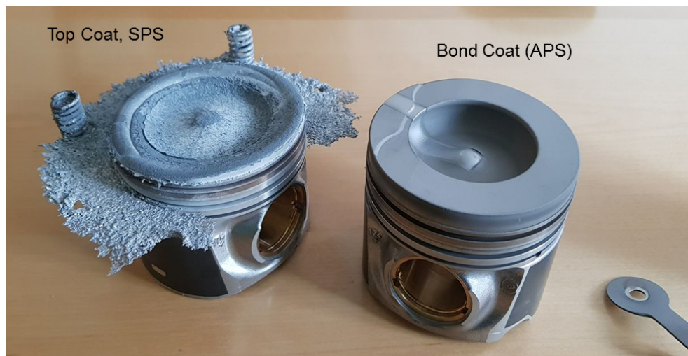
Figure 23. Spray trials with bond coat (right piston) and suspension plasma sprayed YSZ (left piston).
