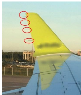
Figure 3.13: Dischargers installed on airplane wings.
