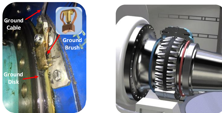
Figure 3.4: Typical ground brush and wind turbine main bearing.
