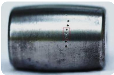
(a) Craters on bearing roller
