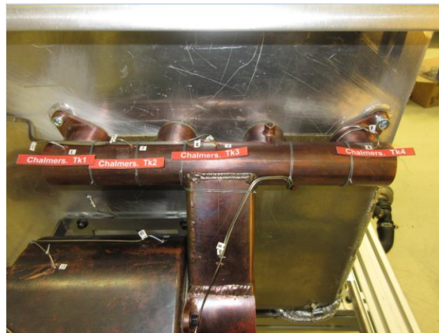
Figure 3. An example of embedded thermocouples installation.
