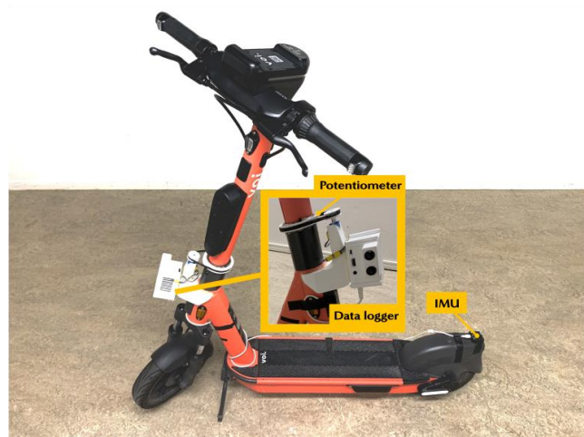
Figure 2. Data loggers installed on the four vehicles used in two experiments.
