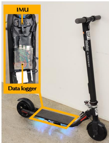
Figure 2. Data loggers installed on the four vehicles used in two experiments.
