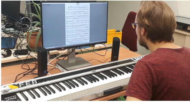
Figure 2: Apparatus showing the MIDI keyboard, two loudspeakers and a monitor with attached eye tracker connected to the stimulus and recording laptop (left).
