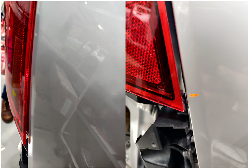
Figure 11. Fitment issues, left Flush and right Gap.
