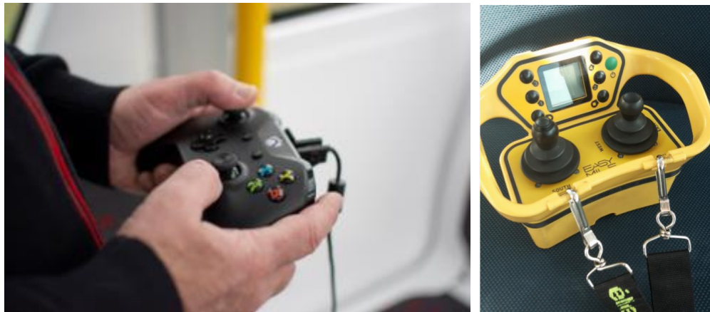
Figure 23. Manual control unit for the shuttles. Connected by cable or by remote configuration
