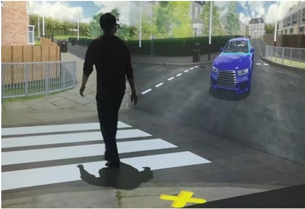
Figure 14 Interaction between the pedestrian at the zebra crossing and the AV approaching from the right, with the eHMI on, in the HIKER lab. The yellow X indicates the pedestrian's starting position.
