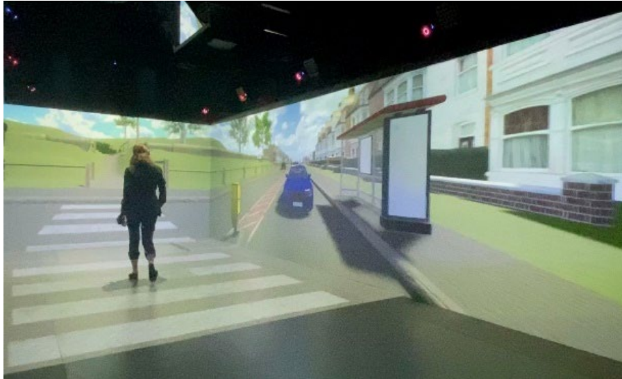
Figure 7 the pedestrian's view of the vehicle in the pedestrian lab: the pedestrian is walking on the zebra crossing and the subject vehicle is to their right.
