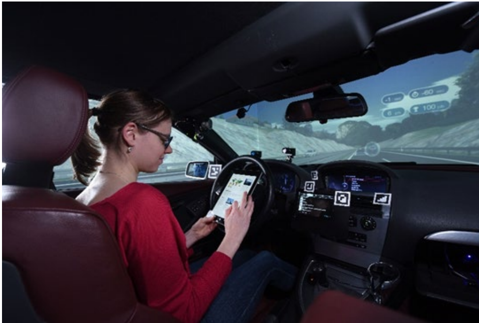
Figure 12 Automated driving simulation at the Chair of Ergonomics (TUM)
