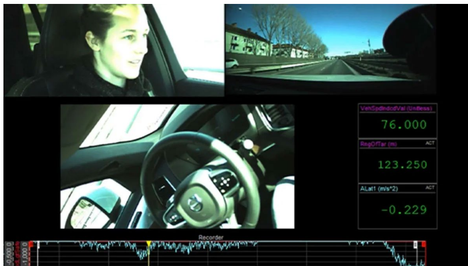
Figure 5- Instrumented vehicle to collect naturalistic driving data (published with author's permission)
