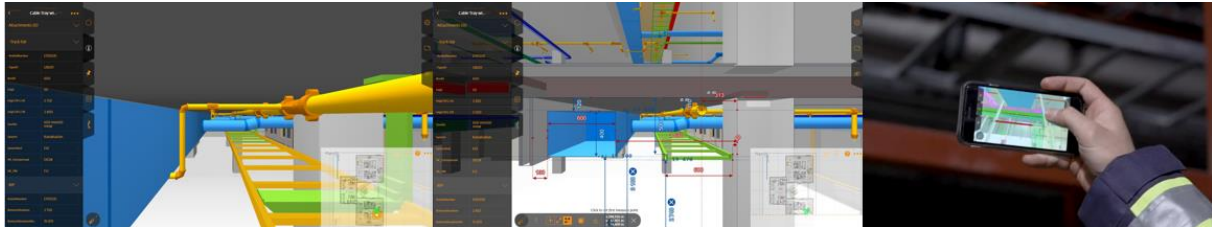
FIG. 4: Site workers can use mobile devices to navigate in either 2D or 3D to their current work area and create unlimited sections and measurements (Image from case projects: Lumi and Celsius).
