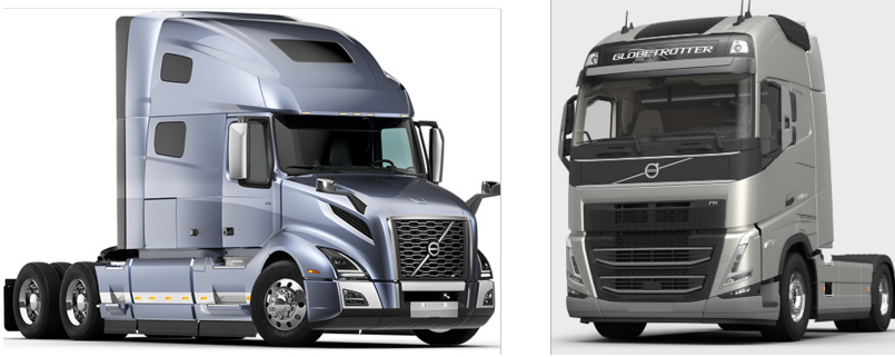
Figure 4.3: Variation in cab geometry in Volvo Truck products offered in North America (left) and Europe (right)
