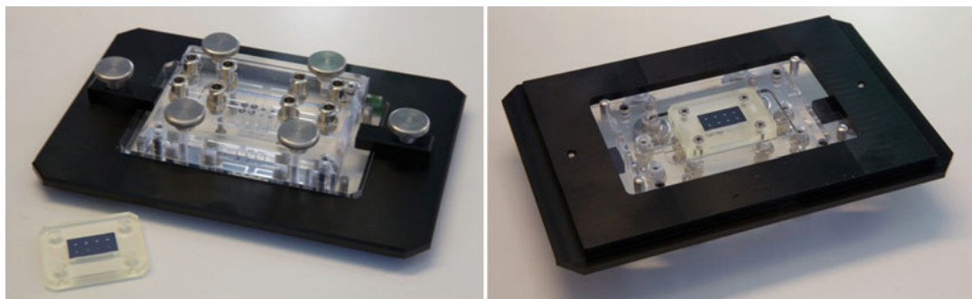
Fig. 1 Example of chuck for mounting samples. Modular design with separate parts for frame and fluidics. The device chips are mounted in plastic holders for easy handling. Eight reservoirs linked by o-rings to the fluidic access holes on the chip. Reservoirs are individually addressable by pressure and electrical connections. (Left) Top view. Device chip is not mounted. (Right) Bottom view with mounted device chip
