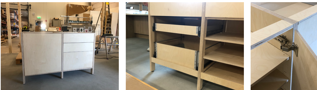
Figure A4. Prototype cabinets showcasing the plywood construction based on flexible furniture connectors.
