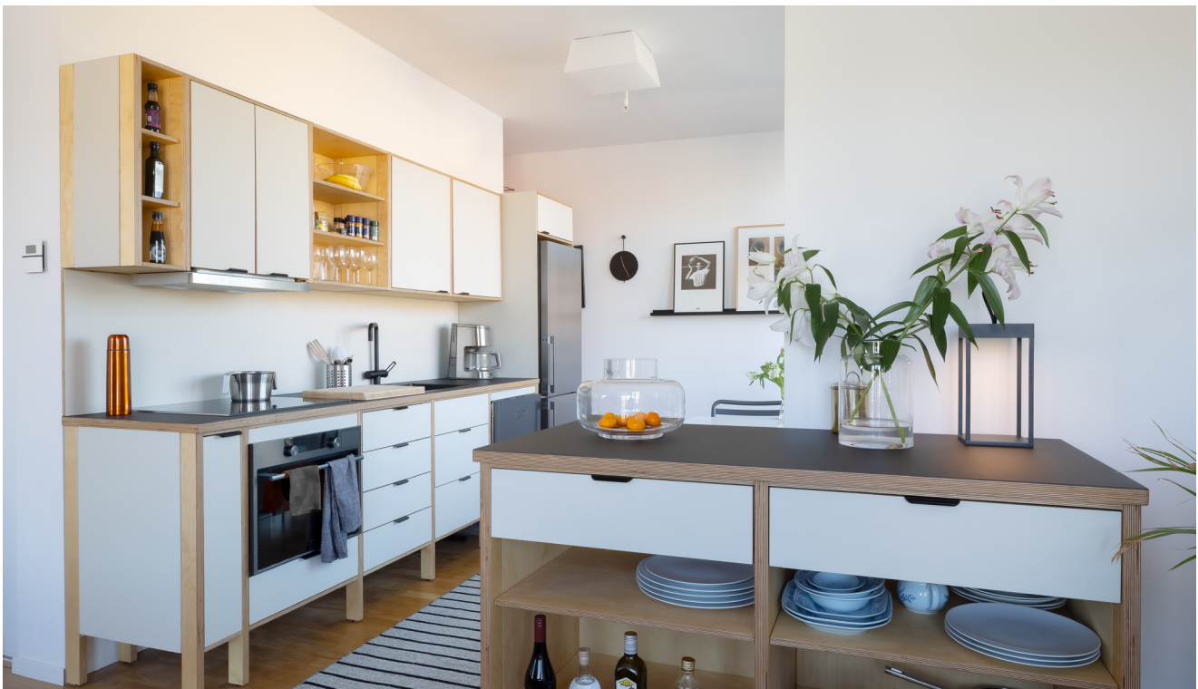
Figure A5. Prototype kitchen installed in living lab, featuring a modular plywood construction and moveable kitchen island to adapt to changing social settings and functional demands.
