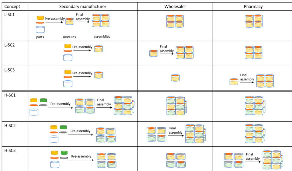
Figure 5. The nature of product variety conceptually illustrated for modular product designs for each SC stakeholder for SC archetype.
