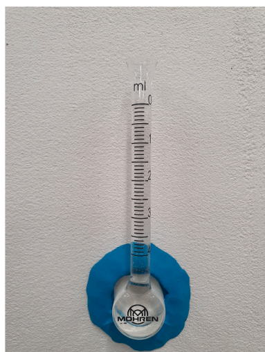
Fig. 8. Karsten tube affixed to the surface of a specimen. A steady water pressure created by 100 mm column corresponds to a wind pressure (1100 Pa) at velocity of 43 m/s.
