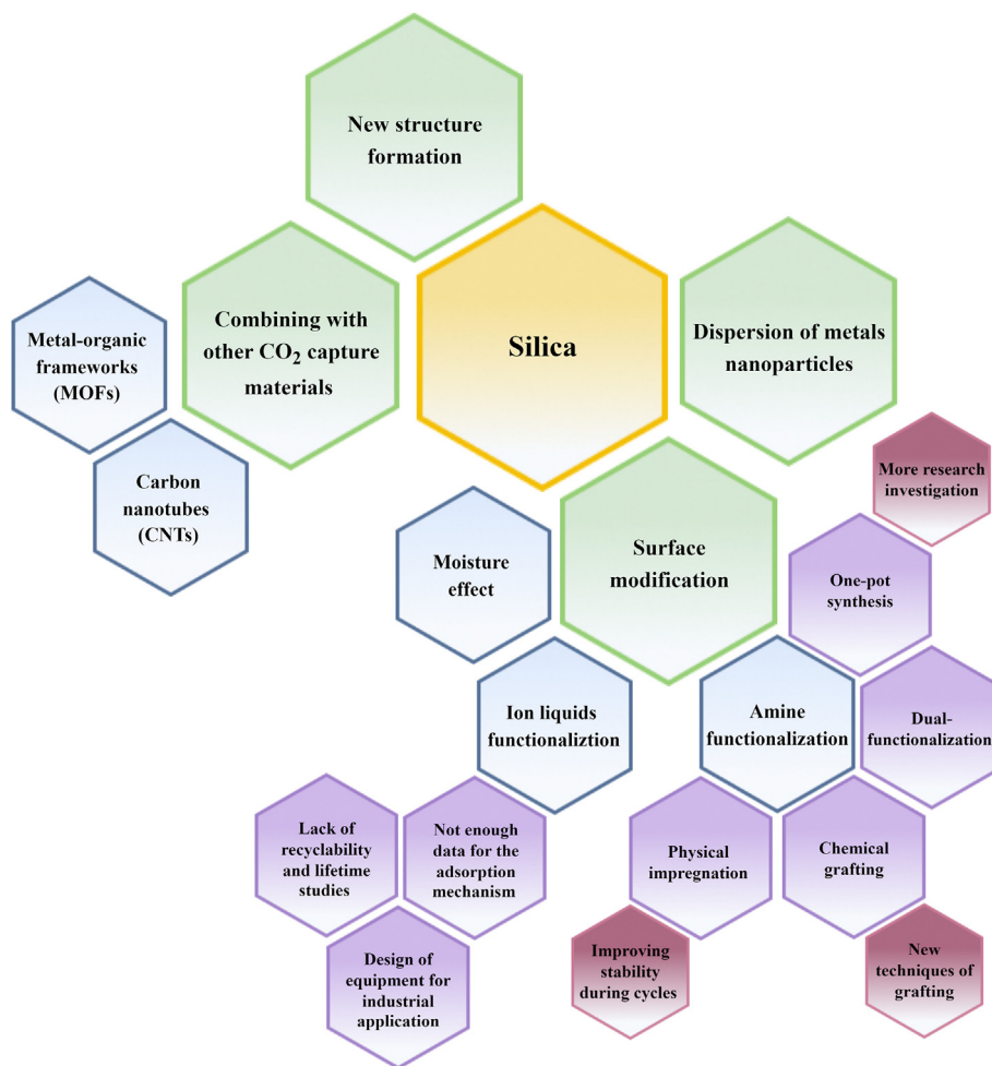
Fig. 6. The modification strategies and research directions of silica-based adsorbents.
