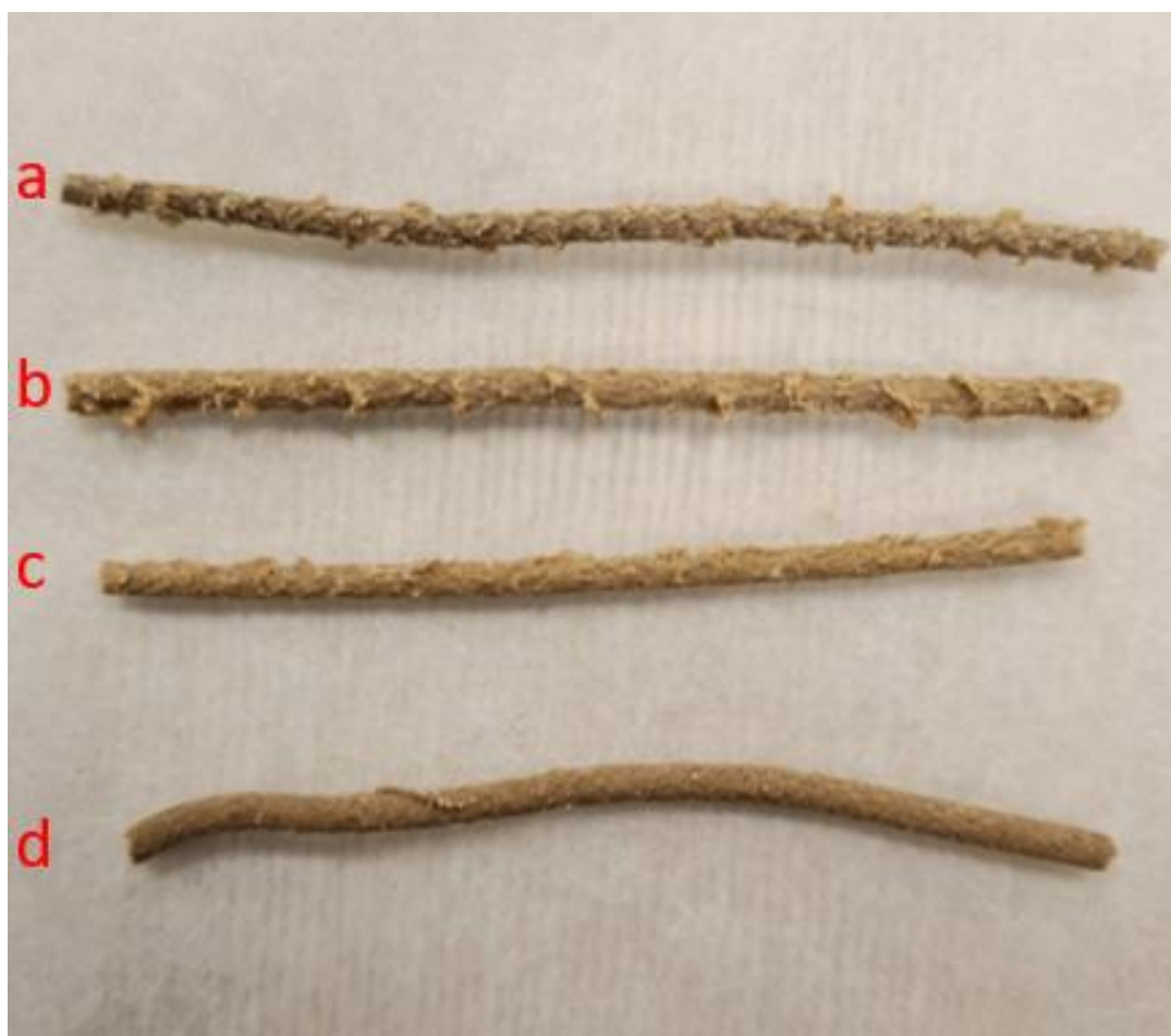
Figure 11. A visual impression of filaments composed of a) PP-TMP b) PP-TMP AKD Hex c) PP-TMP AKD Lau and d) PP-TMP AKD St, as compounded for 10 minutes and extruded at 150 kN and 190 °C.
