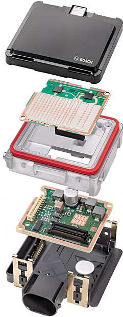
Figure 2.4: Exploded view of the Bosch RADAR sensor [51].
