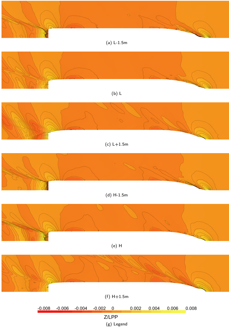
Figure 14: Wave pattern contours for different loading conditions at 17kn
