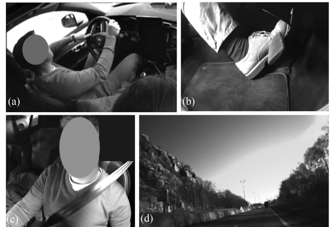
Fig. 4. Video views used for manual coding show: (a) driver's upper body and hand placement, (b) driver's feet and brake/accelerator pedals, (c) driver's face and eyes, and (d) the forward roadway.
