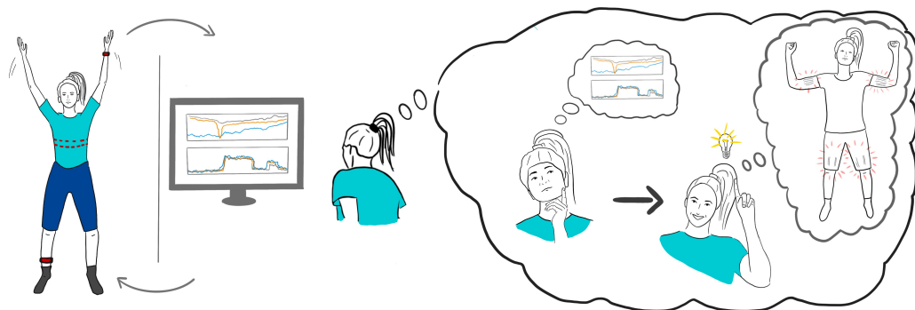
Fig. 1. A typical high-intensity interval training (HIIT) session with REPLAY (Reflective Physical Activity). In between performing high-intensity exercises, users study recorded physiological signals from their body-worn sensors (heart rate and movement). Our work showcases how this form of in-session reflective feedback provides users with the means to better understand the effects of fast-paced physical activity on their bodies.
